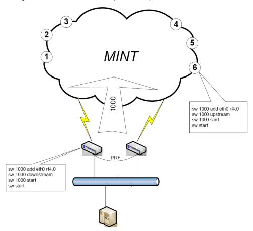
Entire downstream (from server to camera) traffic, if any, is transferred in group number 1000 in which all the nodes are located. But upstream flows from each camera are transmitted directly to the nearest hub of the group.
