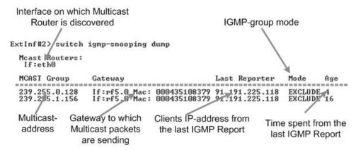
Parameter "detail" allows seeing detailed information on Multicast-subscribers.
