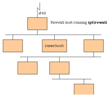
All subnets of an inner network, including a host address innerhost, are owned by the one network (or a network group). Let's imagine that outer network has no hosts which are within the range set up for the inner network. Therefore, all the packets that are accepted via rf5.0 interface of the router with firewall run on it and have the source address which is in the range of addresses of the inner network must be blocked. The following command can perform this action:
