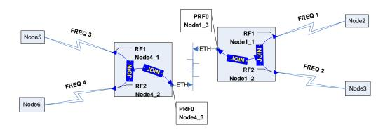
In this example we have joined several distributed (possibly even geographically distributed) network segments. Combining "joins" for different radio interfaces and pseudo radio interfaces the network will obtain a good number of alternative paths in any direction thus providing with the best delivery quality and less bottlenecks.
