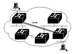
There are several approaches to build tunnels. One of these, IP into IP Encapsulation (described in RFC 2003), is implemented in OS WANFleX. This technology is used, for example, in Cisco Systems routers, and is a subset of the IPSEC protocol supported by several operating systems.
