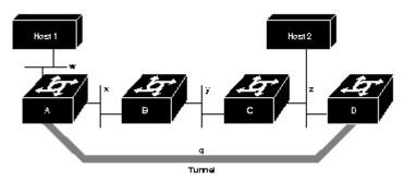
Tunnels also solve the problem of using common transport media in a public network so that different clients could be provided with services by several providers. It means that a client can be connected by a tunnel to a specific provider, to be serviced by that provider, irrespective of the client's connection point to a common transport network.
