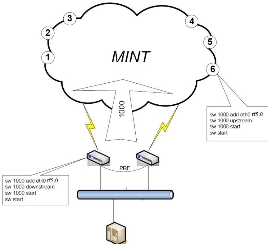
Downstream (from server to camera) traffic, if any, is transferred in group number 1000 in which all the nodes are located. But upstream flows from each camera are transmitted directly to the nearest hub of the group.
