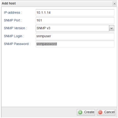
Figure - Adding the device
