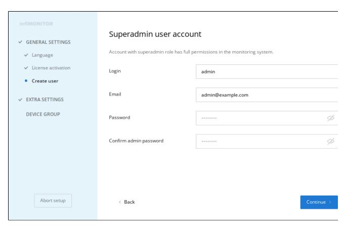
Fill in the required fields and click on the "Continue" to proceed the creation of SNMP profiles and Email settings. These settings are not required to start the monitoring system, so they can be skipped and configured later. You can read about how to do this in the "System Configuration" section.
