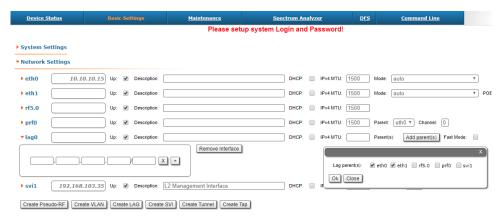
3. Select LACP (Standard or Fast mode). "Standard" LACP fully complies with the standard IEEE 802.3ad. "Fast" LACP uses only with InfiNet Wireless devices and increases efficiency and performance compared "Standart" mode.
