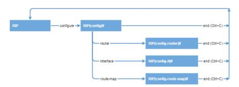
Figure - The transition scheme between different modes of CS
