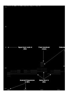
Spectrum analyzer output
