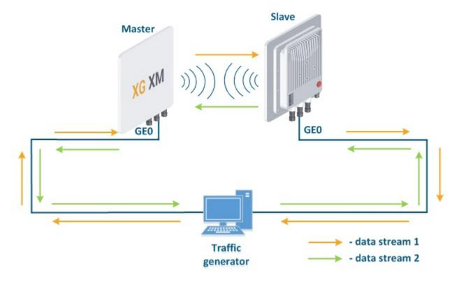
Figure - Bidirectional throughput test
