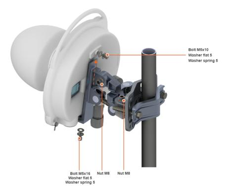
Mounting is carried out on a pole with a diameter 30 ... 85 mm. There are also possible options for mounting on a wall or pole with a diameter more than 85 mm.
