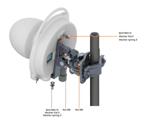
Mounting is carried out on a pole with a diameter 30 ... 85 mm. There are also possible options for mounting on a wall or pole with a diameter more than 85 mm.
