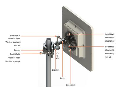
Mounting is carried out on a pole with a diameter 30-85 mm. There are also possible options for mounting on a wall or pole with a diameter more than 85 mm.
