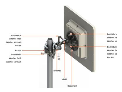
Mounting is carried out on a pole with a diameter 30-85 mm. There are also possible options for mounting on a wall or pole with a diameter more than 85 mm.
