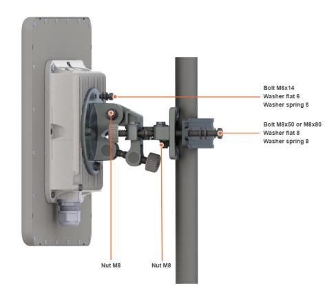
Mounting is carried out on a pole with a diameter 30 ... 85 mm. There are also possible options for mounting on a wall or pole with a diameter more than 85 mm.
