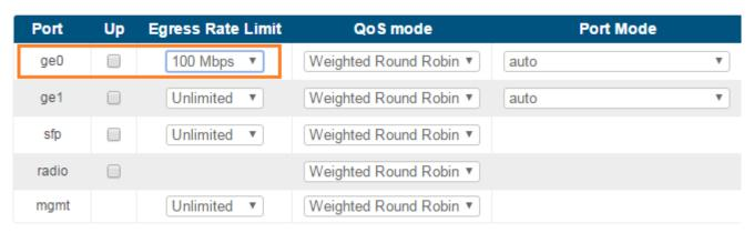
Figure - Configuring per-port egress rate limiting
