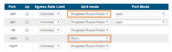
Figure - Configuring the packet scheduling algorithm
