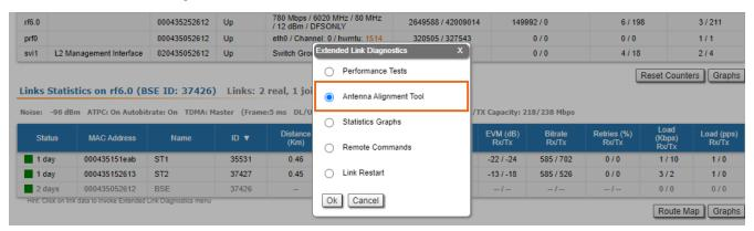
The team at the antenna which has the highest gain will click on the "Start Test" button and start to change the azimuth slowly while watching the signal indicators
