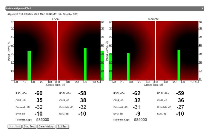
As soon as the antennas have been precisely alignment, set the "auto" option for Tx power and bitrate at both units and select values in accordance with the EIRP limitations.
