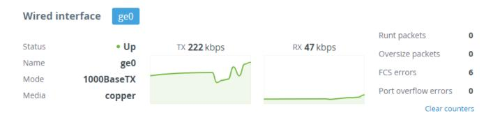
In the "Wired interface" section, you can monitor the wired interface status and its traffic load for reception and transmission. The wired interface statistics is on the right side and can be reset by clicking the "Clear counters" button. Pay attention to the FCS errors number which indicate a violation of data integrity during transmission over the wired segment. Also, the problem can be caused by a queue (port) overflow or inappropriate frame size (runt and oversize).
