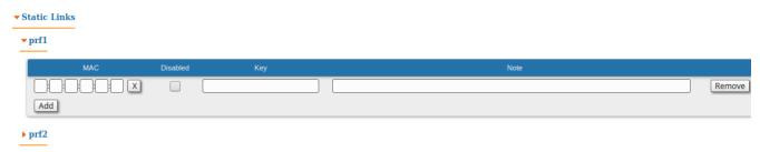
By clicking the "Add" button, you create a new fixed link to the unit. By clicking the "Remove" button, you can delete an already created fixed link.
