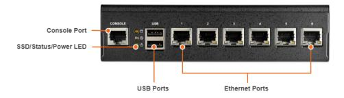
• Console port - RJ-45 console port to connect to a computer terminal for diagnostic or configuration purpose.
