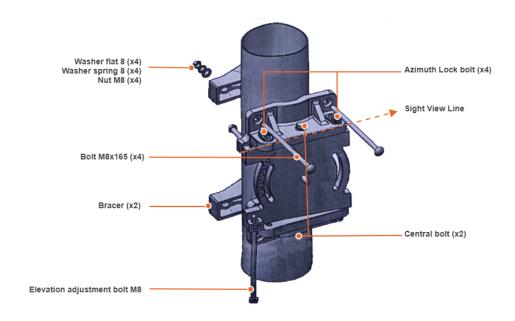
Step 1: Put Bolts M8x165 to its sockets, attach to the mast and assemble Bracers on the bolts. Put the Nuts M8 and Washers 8 (flat and spring) on the bolt without fastening.
